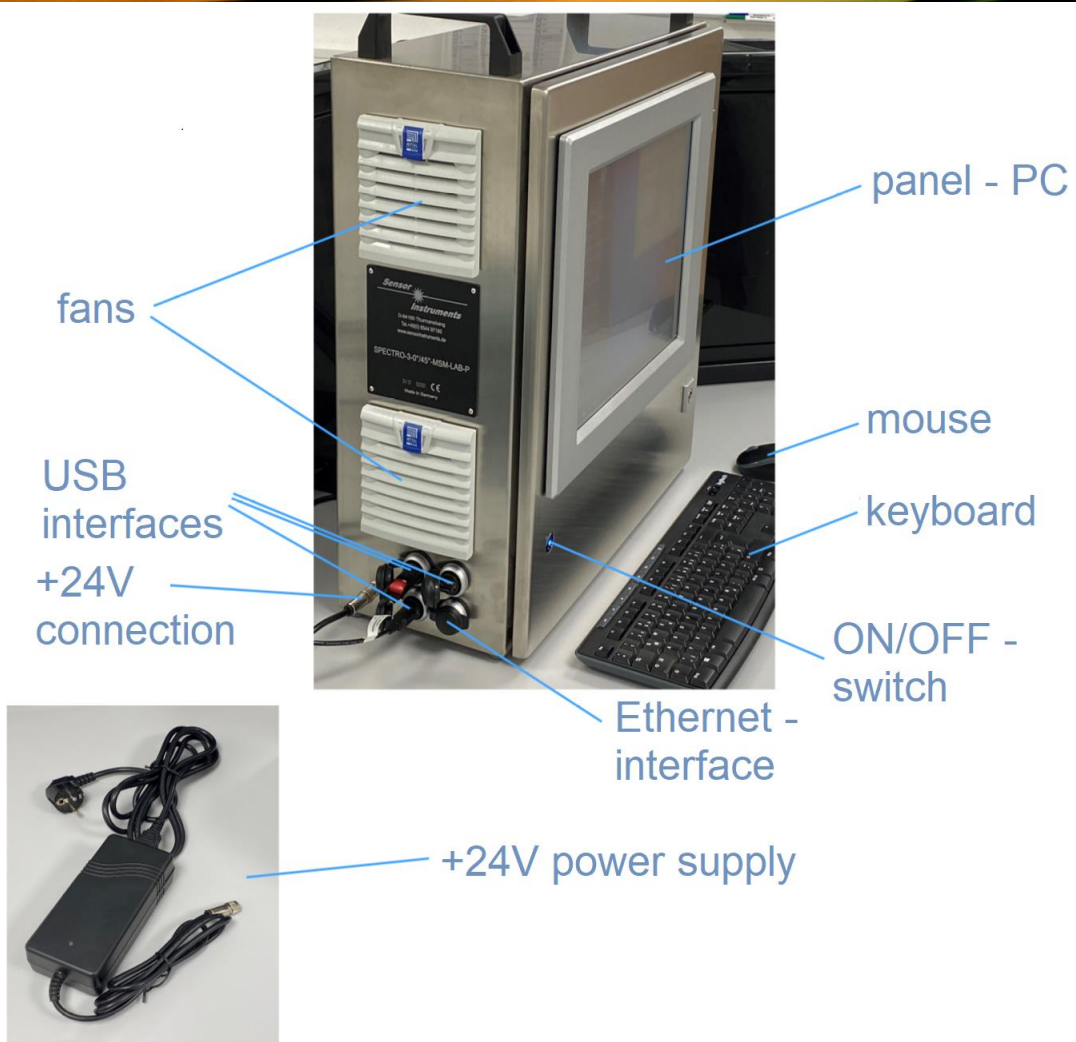
Electrical and mechanical interfaces of the lab colorimeter SPECTRO-3-0°/45°-MSM-LAB-ANA-P
