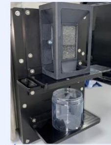
Calibration card holder, holder for pellet samples, pellet hopper with sight glass, slider
